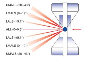
FIGURE 39-10 Light scatter measurements from the Unicel® DxH 800 flow cell. The upper median angle light scatter (UMALS) and lower median angle light scatter (LMALS) detect the cell's granularity and membrane topography. The axial light loss (AL2) evaluates cellular transparency and the low-angle light scatter (LALS) is used as a cellular complexity index.
