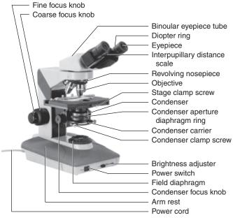
FIGURE 37-2 Basic components of the compound microscope.
