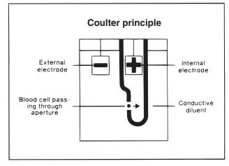
FIGURE 39-1 Coulter principle. Increased electrical resistance, or impedance, occurs when the poorly conductive blood cell passes through the aperture.
