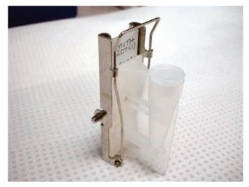
FIGURE 30-7 Cytocentrifuge slide assembly with disposable dual chamber cytofunnel.
