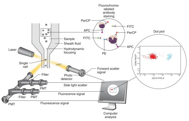
**FIGURE 40-1** Flow cytometer. The cells in the specimen are stained with fluorochrome-labeled antibodies and separated into single cells that pass in front of a laser light source. Scattered and emitted light are detected with photodectors and photomultiplier tubes (PMTs), undergo computer analysis, and are displayed as dot plots.
